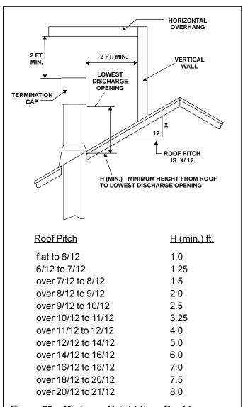
Figure 26. Minimum Height from Roof to Lowest Discharge Opening
